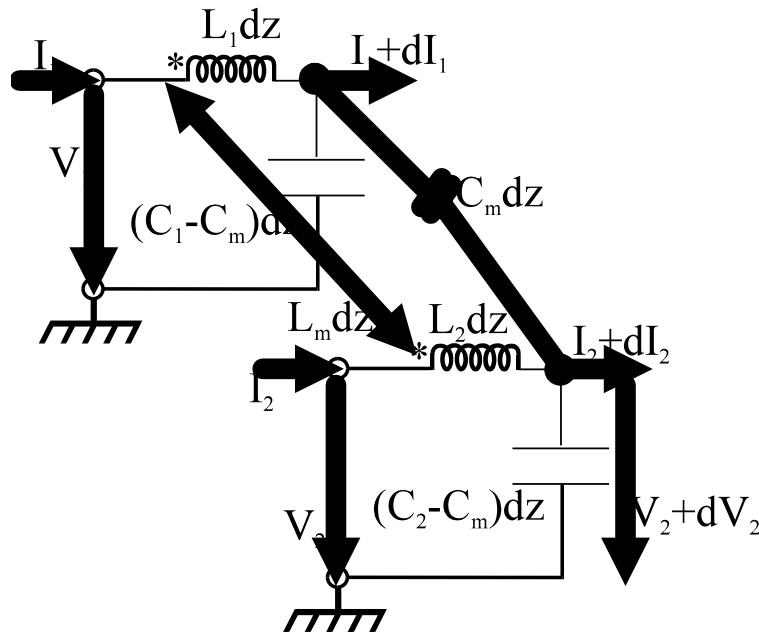
$$\left\{ \begin{array}{l} -\frac{dV_1}{dz} = j\omega L_1 I_1 + j\omega L_m I_2 \\ -\frac{dV_2}{dz} = j\omega L_m I_1 + j\omega L_2 I_2 \\ -\frac{dI_1}{dz} = j\omega C_1 V_1 - j\omega C_m V_2 \\ -\frac{dI_2}{dz} = -j\omega C_m V_1 + j\omega C_2 V_2 \end{array} \right.$$
